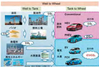
図 Tank to Wheel と Well to Wheel
